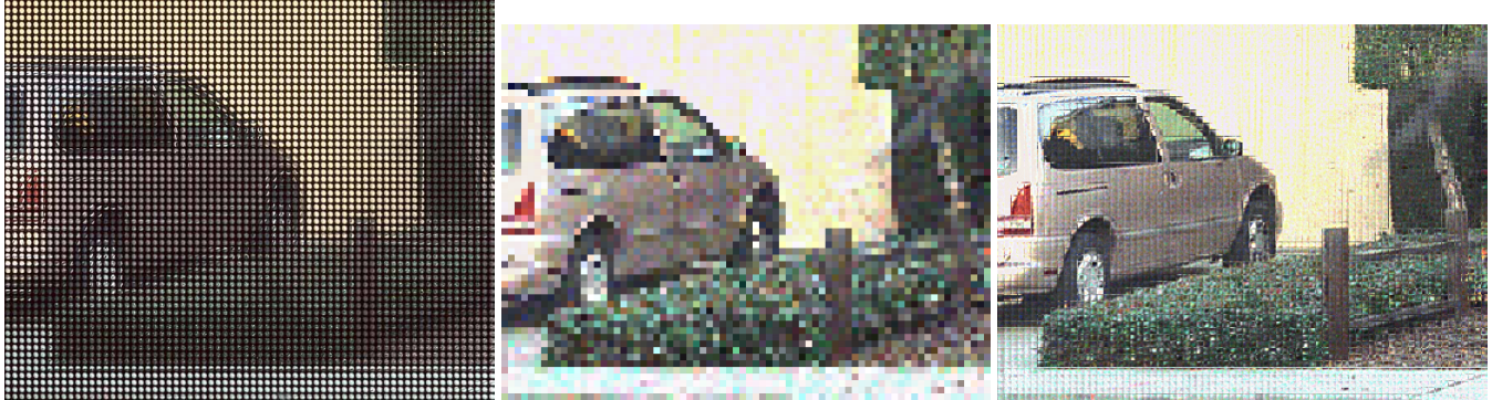
Figure 1: Example of lightfield, normally rendered image, and full-resolution rendered image.
