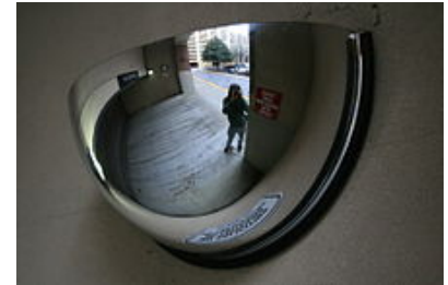
Convex mirror lets motorists see around a corner.
